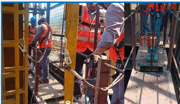
Wire Rope Tester Instrument fixed for scanning of cage winder ropes at Mahagiri Mines (Chromite), Indian Metal and Ferro Alloys, Jajpur, Odisha
