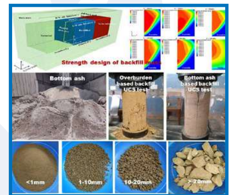
Fig. 2. Studies for backfill required strength design, OB and bottom ash use for underground stope backfilling.
