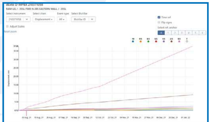
Fig. 17: Readings recorded by an instrumented cable bolts during stoping operation.
