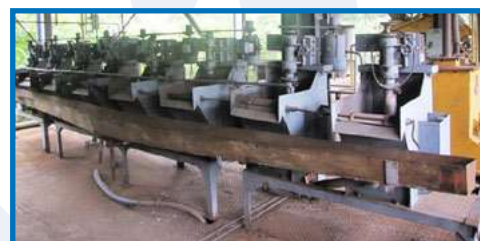
Figure: 400 kg/hr pilot scale flotation plant
