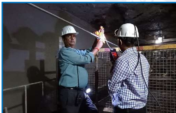
Scanning of haulage rope in progress in Man Riding Chair lift system in Underground mine at Nandira Colliery, Mahanadi Coalfields Limited, Talcher, Odisha
