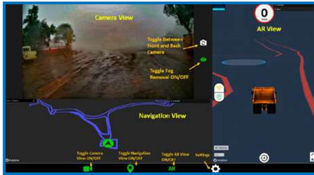
Fig. 3. Integration of V2X, GNSS and radar with a geo-coordinated mine map for real-time display on dashboard screen with split windows
