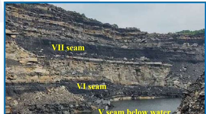
Fig. 11: Highwall mining patch at West Bokaro Mine of Tata Steel Limited where surface structures are present.
