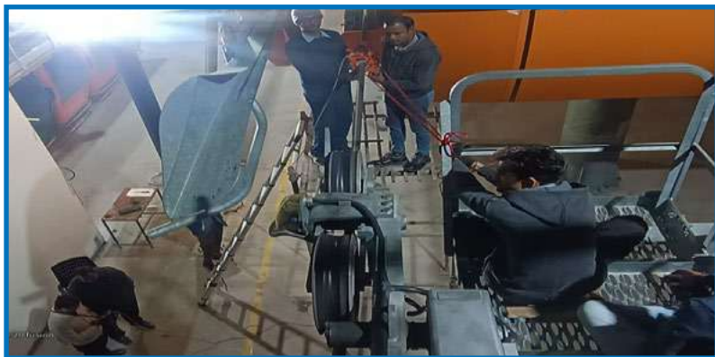
Scanning of Haulage rope in progress for Non-destructive evaluation at Dharamshala Ropeway, H.P.
