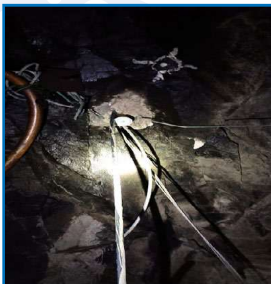
Fig. 21: MPBX installed at the crown pillar.
