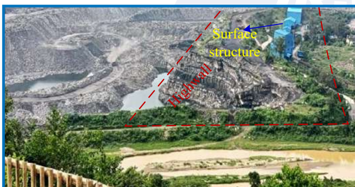
Fig. 11: Highwall mining patch at West Bokaro Mine of Tata Steel Limited where surface structures are present.
