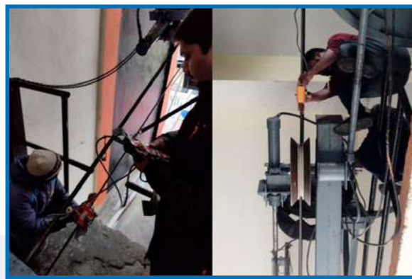
Scanning of haulage rope in progress at LTP and UTP of Bi-cable Passenger Ropeway "Aerial Ropeway" at Nainital, Uttarkhand
