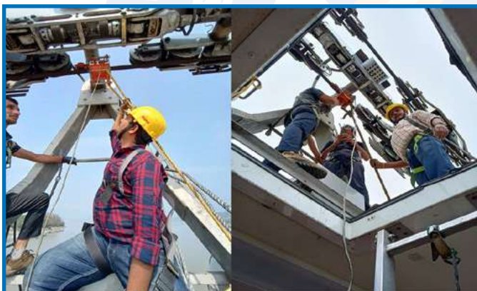
Wire Rope Tester Instrument fixed on the track ropes over cabins of Ropeway across Brahmaputra River, Guwahati
