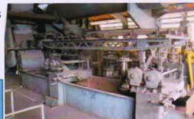
Baum Jig Capacity 20 tph
