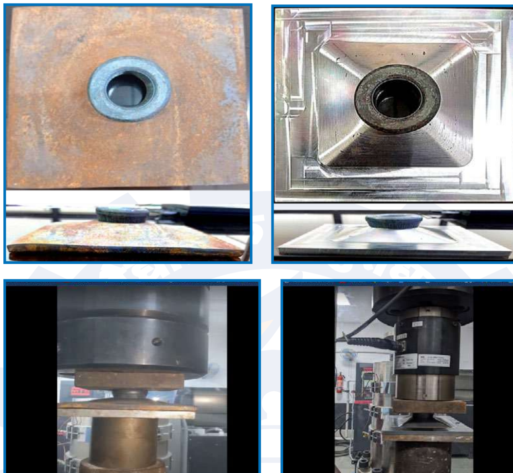
Figure 1: Experiment conducted on the dome and tetrahedron-shaped plates in the testing machine.
