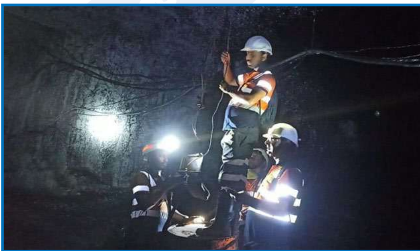
Figure 17: Readings of 4-way roof extensometer taken during mine visit.
