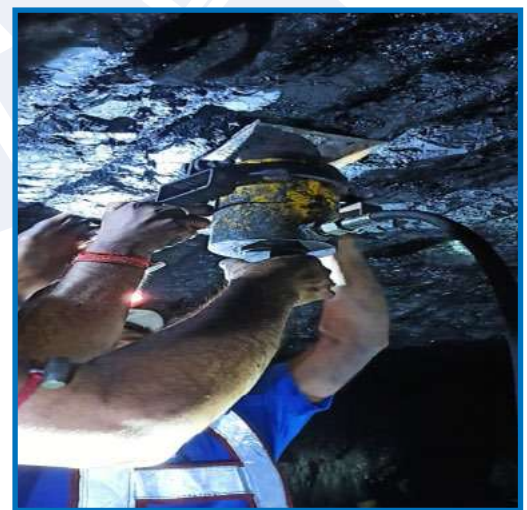
Figure 17: Anchorage testing of roof bolt at the mine site.
