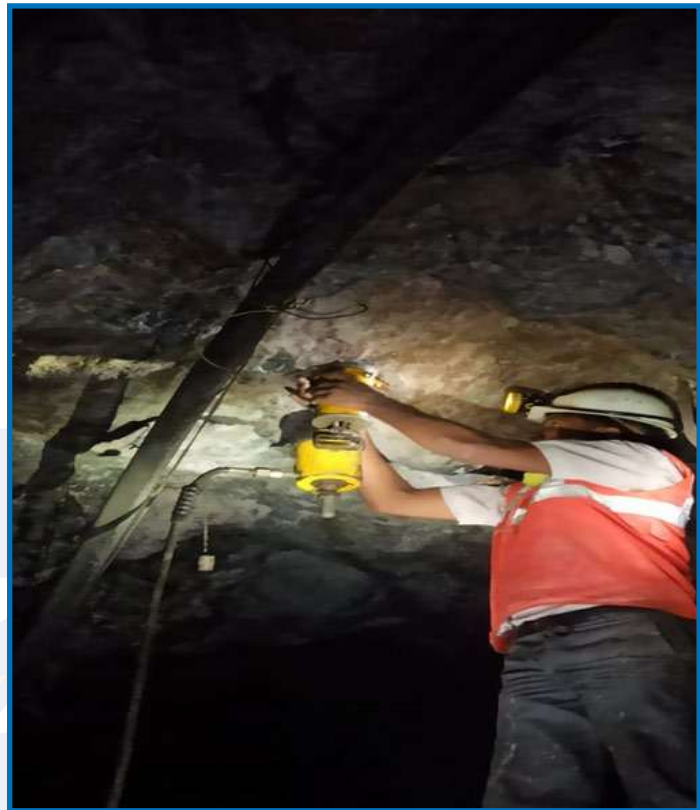
Fig. 24: Anchorage testing of installed rock bolts.
